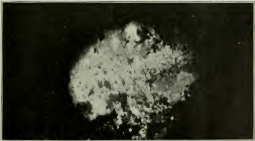
Microphotographs \times 5 diam. Quartz veinlets in ferrodolomite wall rock. Rea Mine. No. 7 is same as No. 6 but as seen with nicols crossed.
